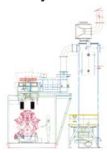
CO and VOC. The uniquely designed catalytic system treats the exhaust from the lean burn Guascor 560GLD, 1.0 MW, natural gas fired, reciprocating engine.
